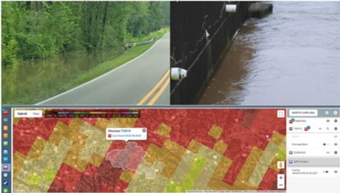
Figure 199: Example of low chord alert and field verification. BridgeWatch links structure elevation thresholds and stream gauge readings statewide monitoring bridge performance and roadway overtopping in real time.
