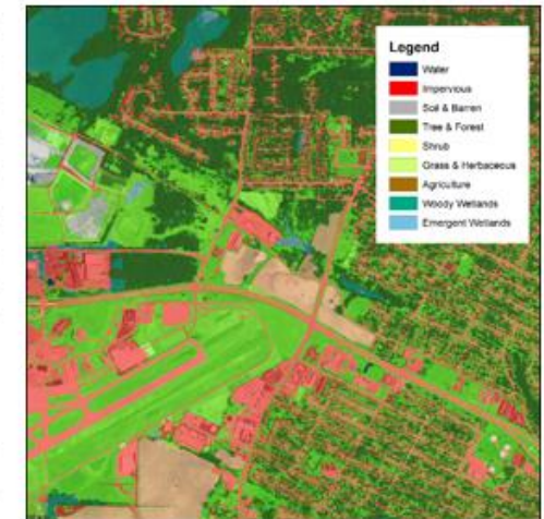
Figure 1 Green Bay, WI urban land cover overlaid on air photo. Each color represents a specific LC class. Note the fine spatial detail showing individual buildings, trees, and roads.
