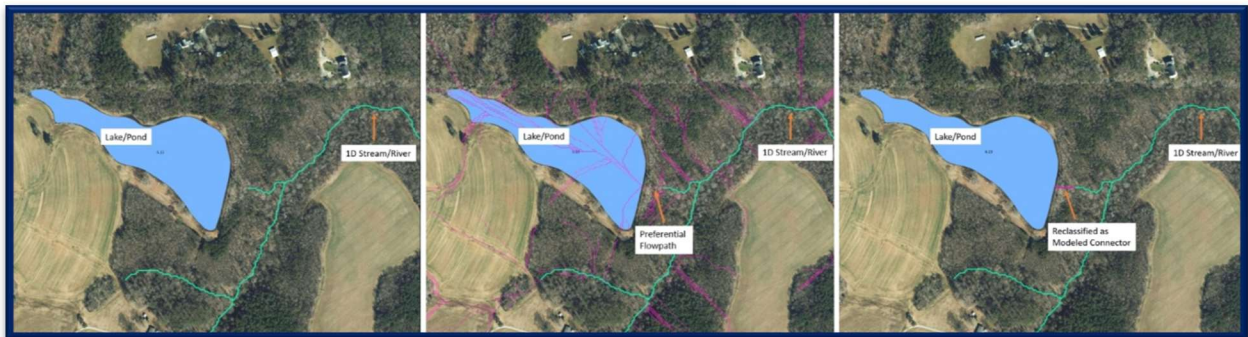
Figure 14. Preferential flow path is reclassified as modeled connector to connect lake/pond to existing hydrography network.
