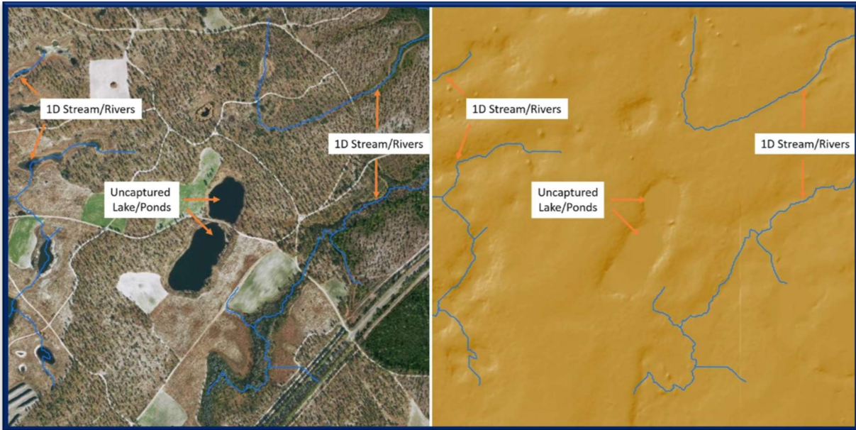
Figure 21. Left- modeled stream network shown on aerial photography of an area of karst topography. Right- hillshade representation of sinkhole area showing ponds with no surface outlet.
