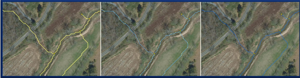
Figure 6. The left image shows the raw rasterized ATLAS data, the middle image shows a smoothed representation on top of ATLAS data, and the right image shows the smoothed data.
