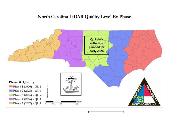
NAD83(2011), NAVD88, and US Survey Foot will be used to collect new LiDAR data in Phases 3, 4, 5
