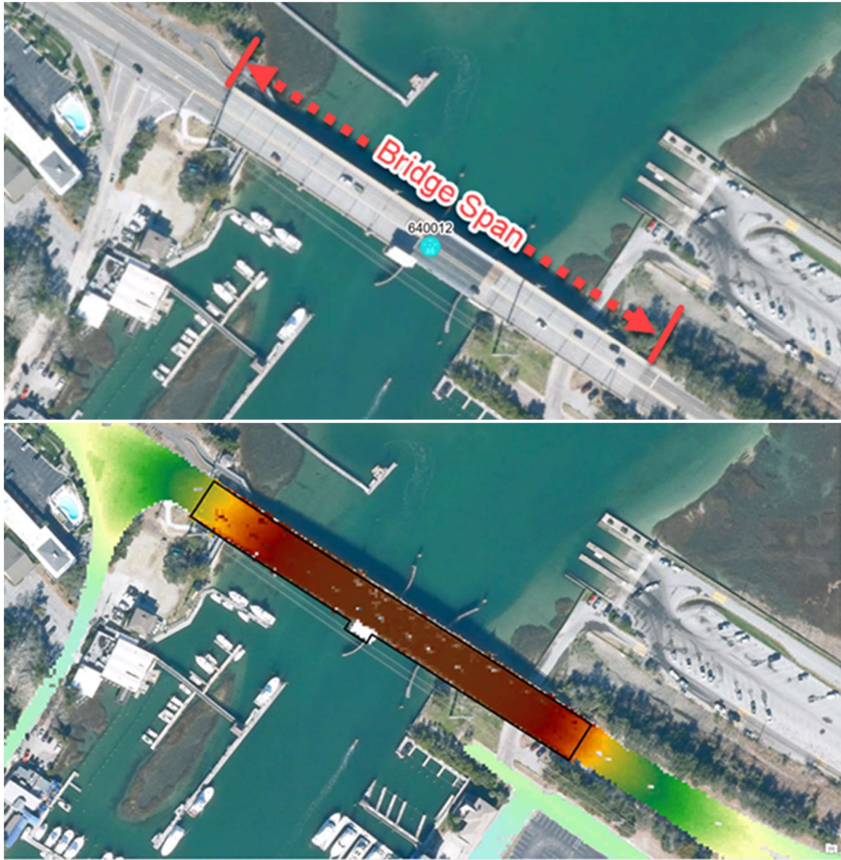
Figure 188: Example of QL-1 lidar data classification of "Road" and "Bridge" used to develop roadway elevation model statewide.
