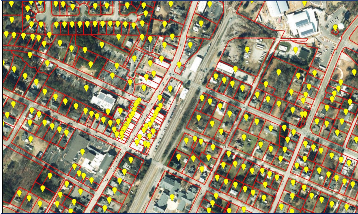
Figure 21. AddressNC compiles a statewide address layer from Next Generation 911 data, producing a dataset that is constantly updated to provide accurate address locations for many applications.
