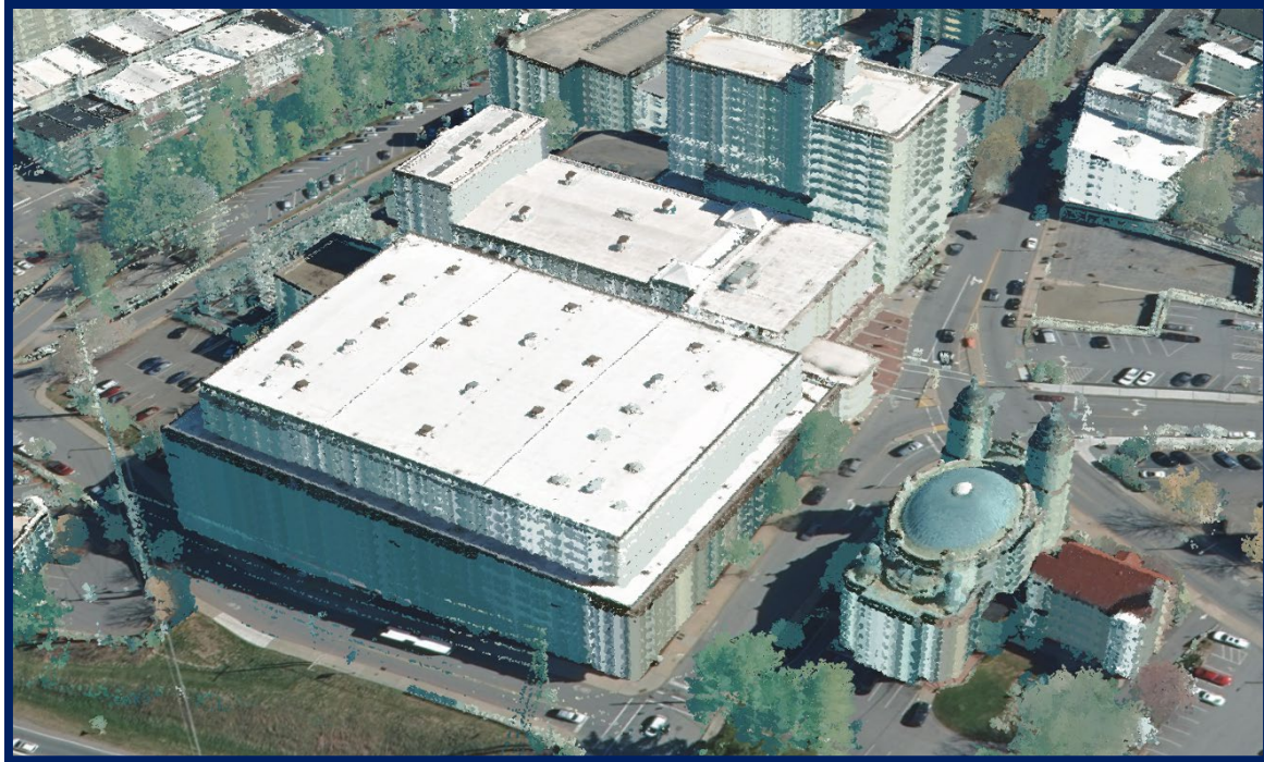
Figure 27. Example of LiDAR point data that has been colorized using NC orthophotography. In this 3D image, notice that LiDAR technology captures not only buildings and vegetation but utilities such as power lines shown in the left forefront. Data visualization by ESRI
