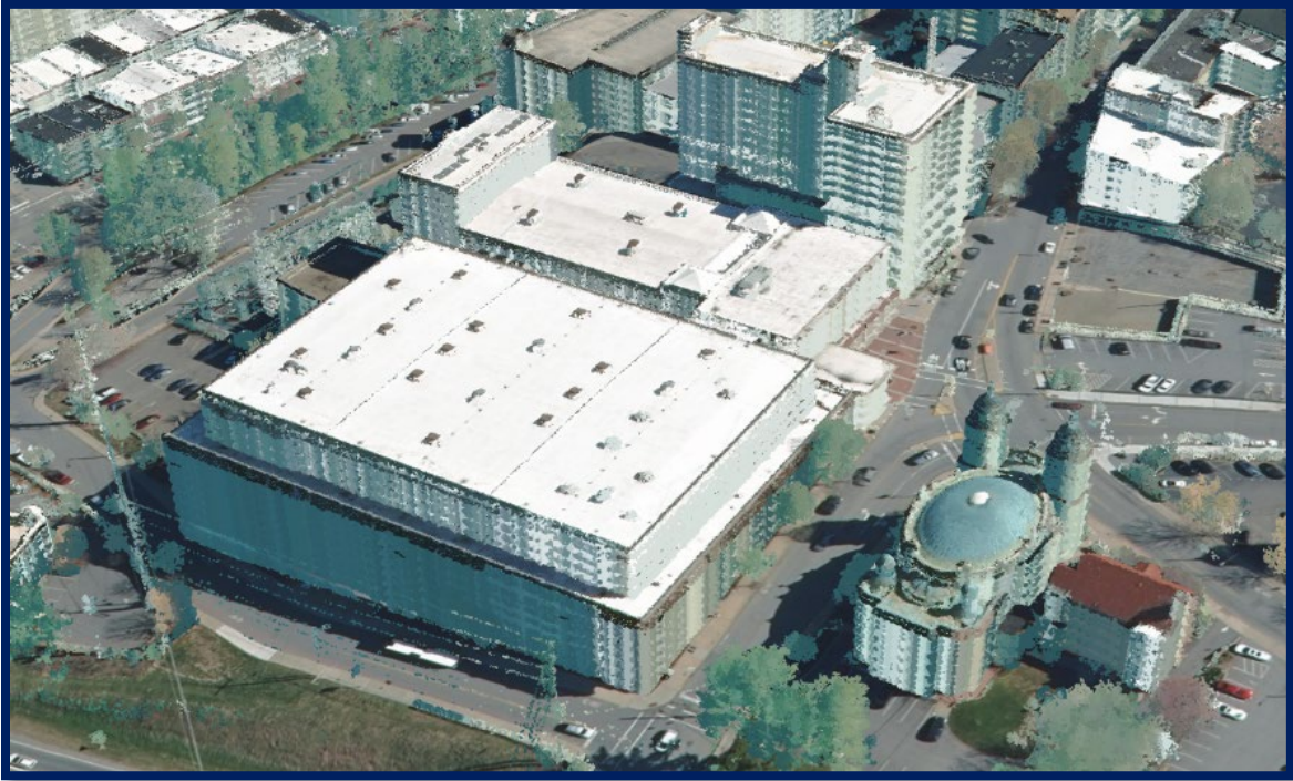
Figure 16. Example of LiDAR point data that has been colorized using N.C. orthophotography. In this 3D image, notice that LiDAR technology captures not only buildings and vegetation but also utilities such as power lines, shown in the left forefront. Data visualization by ESRI.
