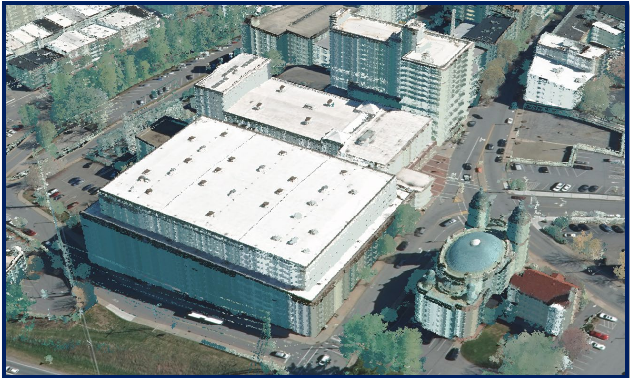
Figure 14: Example of LiDAR point data that has been colorized using NC orthophotography. In this 3D image, notice that LiDAR technology captures not only buildings and vegetation but utilities such as power lines shown in the left forefront. Data visualization developed by ESRI.
