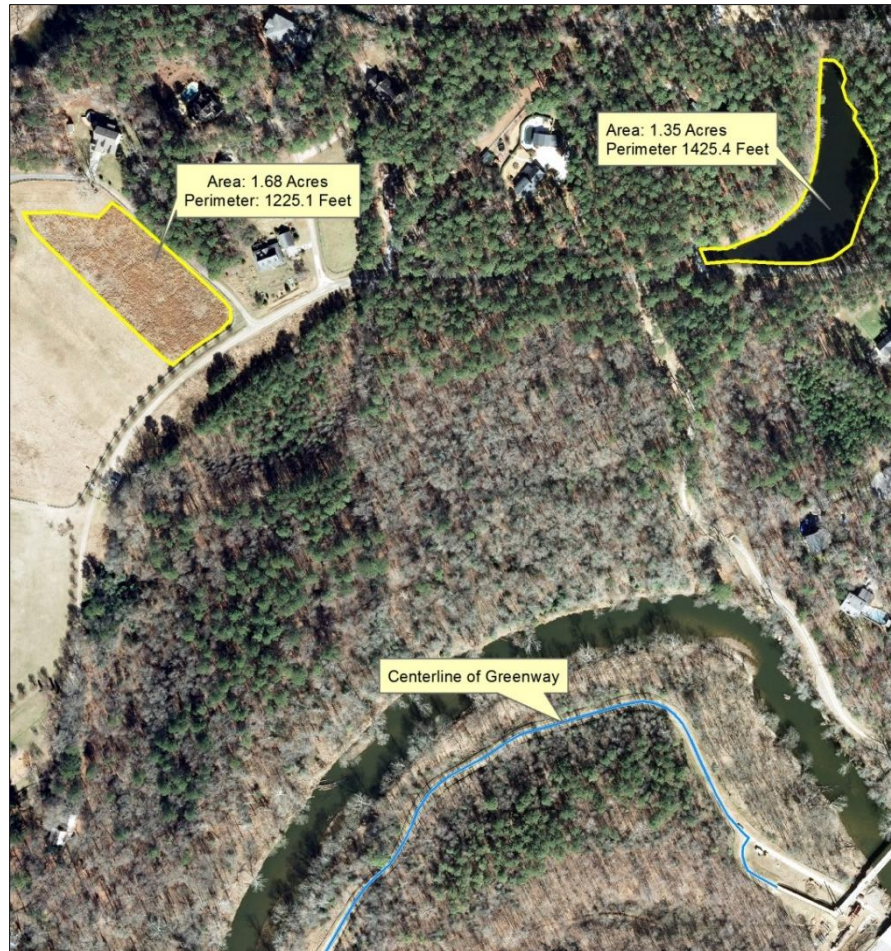
Figure 15. Digitizing without GNSS to create point, line, and/or area features. The example shows a digitized farm field area feature in the top left corner, a digitized pond area feature in the top right corner, and a digitized centerline of greenway line feature in the bottom.
