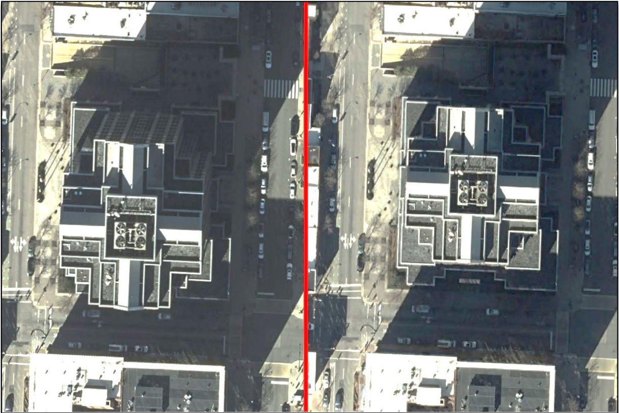
Figure 3: Typical Nadir Orthoimagery (Left) compared with new processing requirements for tall structures (Right)
