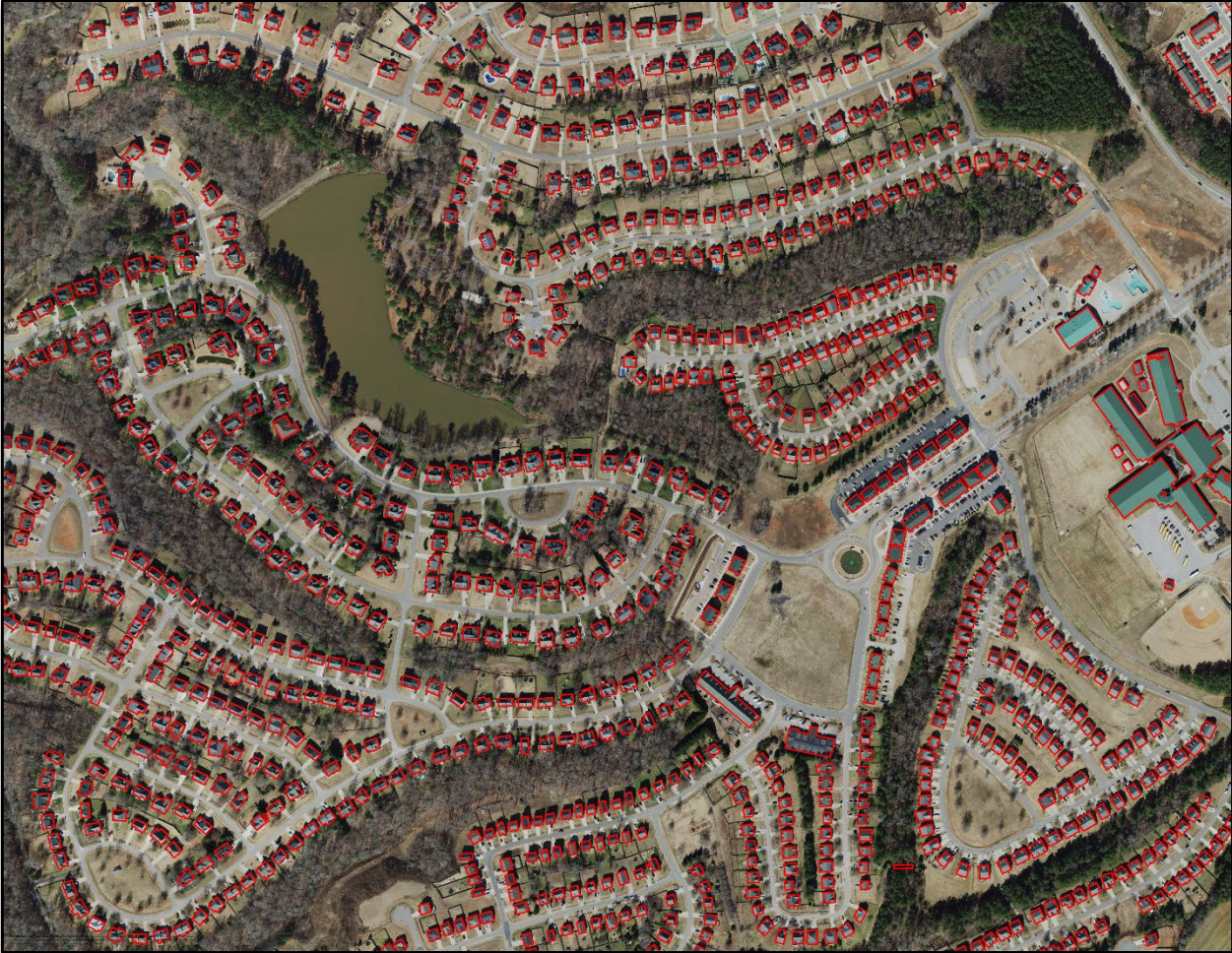
Figure 5: Building footprints extracted from NC Orthoimagery using an Artificial Intelligence Deep Learning Model
