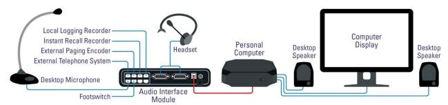
Figure 2-3: MCC 7500E Dispatch Position supports multiple accessories.
