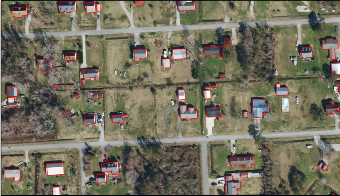
Figure 5: Deep Learning AI Example of Building Footprint Feature Extraction from Orthoimagery
