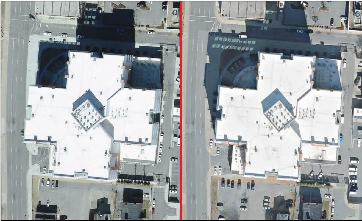
Figure 7: Typical Nadir Orthoimagery (Left) compared with new processing requirements for tall structures (Right)
