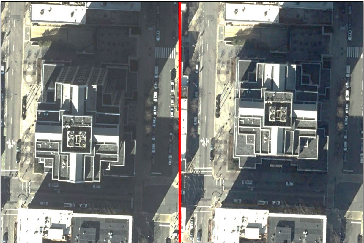
Figure 5: Typical Nadir Orthoimagery (Left) compared with new processing requirements for tall structures (Right)
