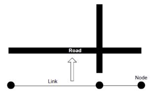
These transportation objects: links, nodes, mile points, calibration points and routes together form networks and linear referencing systems (LRS), and are inherently topological. Transportation networks and LRSs provide information on the feasible paths between specified locations. Once a network or LRS has been created, other
